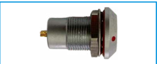
MGG fixed socket, nut fixed, positioning pin (G) or positioning pin (A ... M and R) water-sealed or vacuum-sealed, IP68
