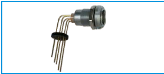
ZCG fixed socket, two nuts, positioning pin (G) or positioning pin (A...F), 90° angled pin core suitable for PCB (rear panel installation)
