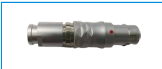
TFA Standard straight plug, cable clip fixed cable, internal parts to prevent cable rotation, sheath to prevent cable bending.
