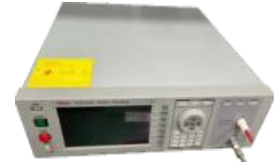
High voltage test machine
