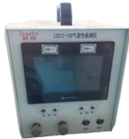
Air tightness testing machine
