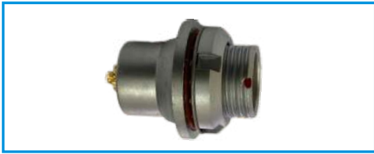
MEG fixed socket, nut fixed, positioning pin (G) positioning pin (A. .. M and R) water-sealed or vacuum-sealed (rear panel installation), IP68
